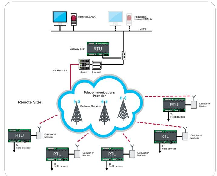
Architecture for remote network using cellular dynamic IP addressing
